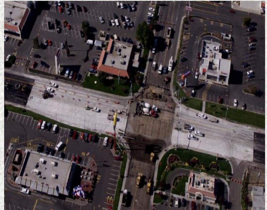
**Design opening strength = 2500 psi. Concrete mix WT (whitopping) from SHA Table 902A provides for minimum compressive strength of 2500 psi in 24 hours!**
