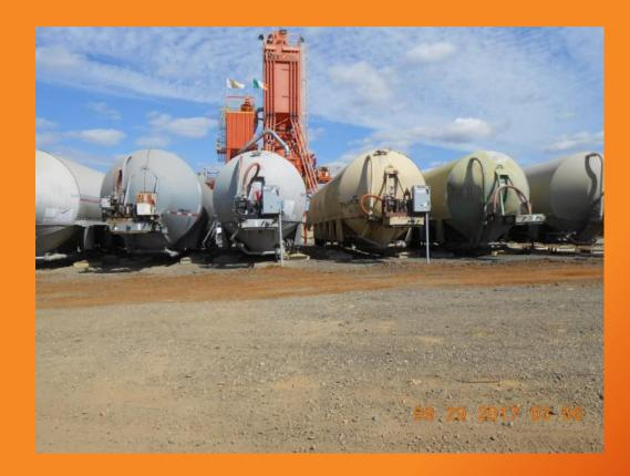
In order to minimize the potential impacts of cement/ slag delays, we installed six "pigs" (bulk cement containers). This would give us a storage capacity of 460 Tons of cement and 450 tons of slag.
