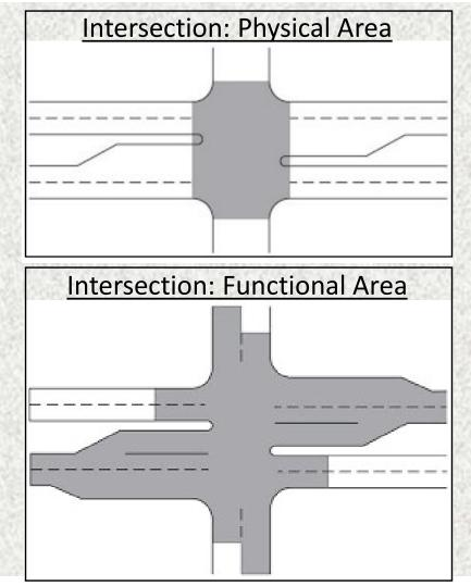
Note 1: Physical area carries the combined traffic from both roadways. Therefore, thickness design must account for both.
