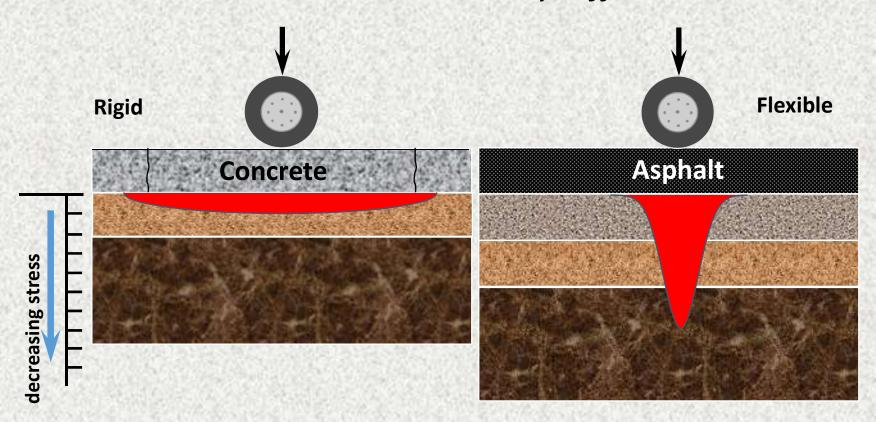
The load capacity parameter for pavements is primarily thickness.
