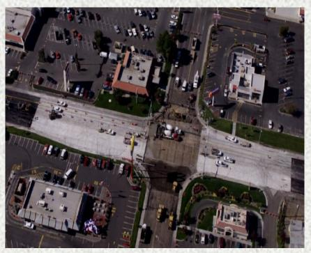
Design opening strength = 2500 psi. Concrete mix <u>WT</u> (whitetopping) from SHA Table 902A provides for minimum compressive strength of 2500 psi in 24 hours!
