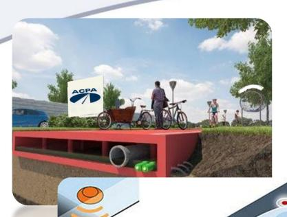
Open and adaptable pavement design options for multifunctionality and ease of utility access
